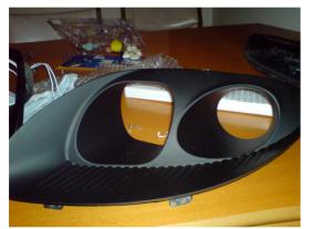
Now get the CCFL rings out and find the matching one to light you are going to work on first (i.e. 80mm is for the smaller hole and 95mm is for the bigger one).
