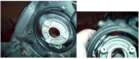
And now just feed the wiring through those gaps that you found, you may have to adjust your light angles to move the reflective parts of the high beam to be able to fit the clip of the wiring through without breaking it.
