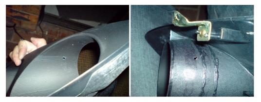
Now drill the hole out by moving the drill head around, till u can just squeeze the clip on the end of the wiring through.
