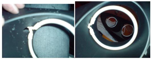
Make sure the ring is in the position you want it to be (and the wiring has been threaded through the hole u just made for it), now apply some super glue to where it touches the casing, once again do this from behind so it wont look so obvious.
