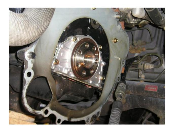
NEXT BIT IS TO CLEAN THE MATING SURFACES OF THE FLYWHEEL AND FIT THAT. IT IS A BIT AWKWARD TO GET IT ON, HOLD IN POSITION, FIT THE PLATE AND WASHER PLATE AND PUT THE BOLTS IN AT THE SAME TIME BUT ACHIEVABLE WITH A BIT OF 'JIGGLING' NOTE THAT THERE ARE 7 BOLTS AND THE ARE NOT EQUIDISTANT. THIS MEANS THE PARTS WILL ONLY FIT ONE WAY AND ALL THE PARTS NEED TO LINE UP OR YOU WON'T GET ALL THE BOLTS IN!! THE FLYWHEEL BOLTS WERE THEN TIGHTENED TO 98NM DOING OPPOSITE BOLTS IN TURN
