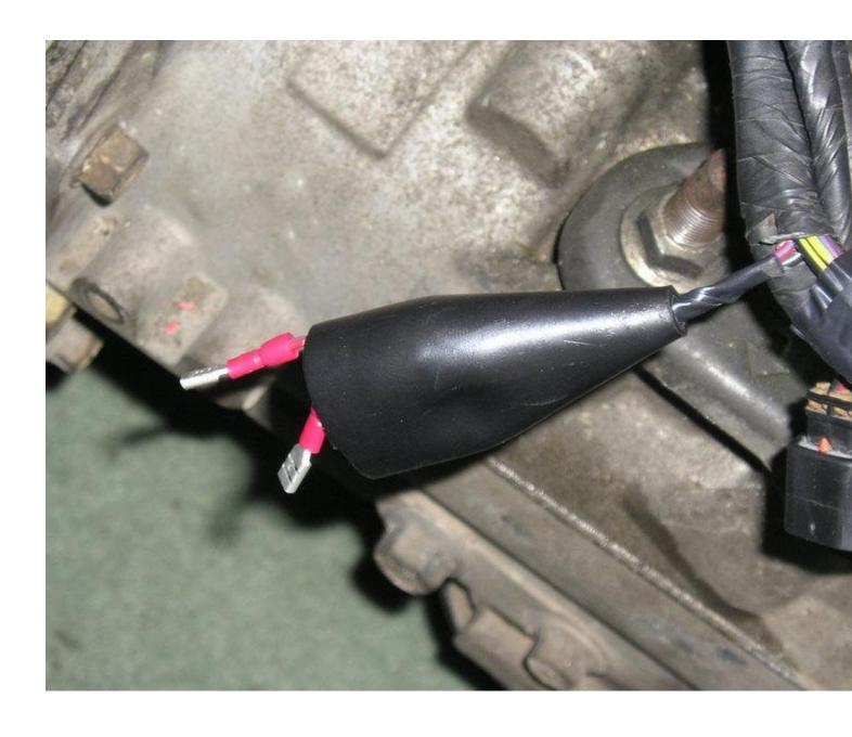
THEN PUSH THE 2 SPADE CONNECTOR ONTO THE REVERSE SENSOR AND SLIDE THE SHEATH DOWN OVER THE TOP LIKE THIS
