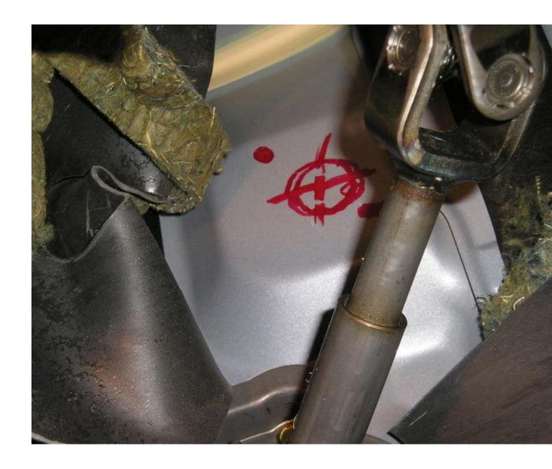
NEXT OFF DRILL THE HOLES. THIS IS A LITTLE TRICKY BECAUSE OF THE ACCESS UNDER THE DASH. I MANAGED TO USE A BATTERY DRILL FOR THE SMALL BOLT HOLES USING A PILOT DRILL THEN OUT TO DIA.9MM THE STUDS ARE DIA.8MM SO THIS ALLOWS FOR A BIT OF CLEARANCE. THE NEXT BIT CUT THE LARGER HOLE WHERE THE MASTER CYLINDER ROD END COMES THROUGH INTO THE PEDAL BOX FROM THE ENGINE BAY. I USED AN ELECTRIC PISTOL DRILL AND A 38MM HOLE SAW. TBH IT FLEW THROUGH THE BULKHEAD.
