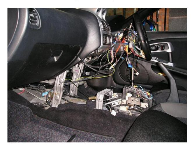
I HAVE UNPLUGGED THE OLD TIP CONNECTIONS AND REMOVED THE 4 BOLTS HOLDING THE SHIFTER DOWN.
