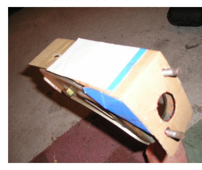
I TRANSFERRED THE CARD TO THE CAR AND BOLTED IT IN PLACE USING THE EXISTING STUD THAT IS ALREADY THERE FOR THE CLUTCH PEDAL BOX. I THEN MARKED OUT THE HOLES READY TO DRILL.
