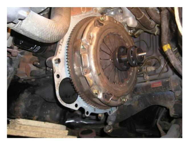
AFTER BOLTING UP THE TOOL WAS REMOVED AND THE COLLET PULLED THROUGH THE SPLINES. THE PRESSURE PLATE BOLTS ON THE CLUTCH COVER ARE TORQUED UP TO 44NM.
